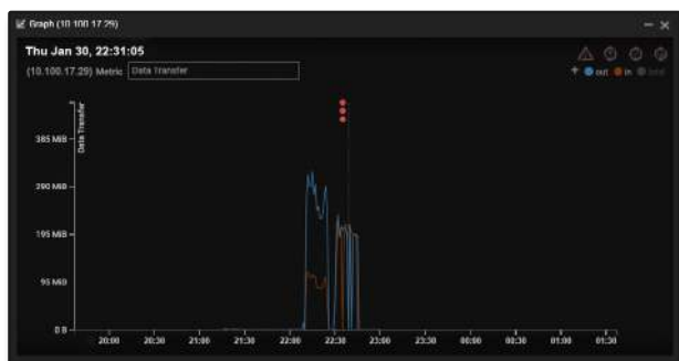
Figure 13: The Threat Visualizer showing a large spike in the number of connections
