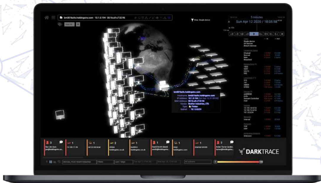
Figure 15: A compromised smart printer and anomalous connections represented with yellow lines
